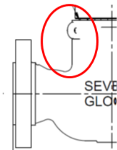
Cast in Lugs – Used on valves greater than or equal to 14" in size. These lugs are a contiguous part of the valve body
