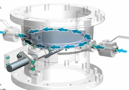
Typical sealant flow path
